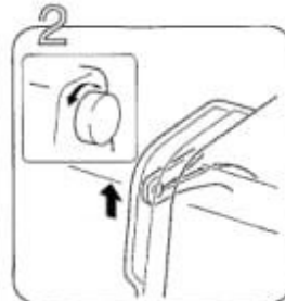
Raise the thread take-up lever to its highest position by turning the balance hand wheel.
