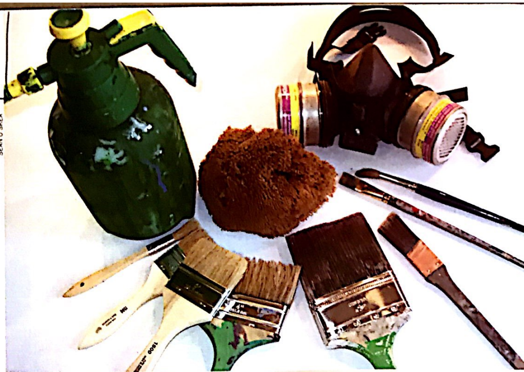
These tools and brushes are all that you need to do most basic scenic painting techniques. Clockwise, from left: a hand-held garden sprayer; a sea sponge; a respirator; a few watercolor brushes; a one-inch Purdy sash-brush; a four-inch hardware-store brush; and a selection of china-bristle "chip brushes."
